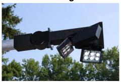
The SSL-45 is a solar powered streetlight. It provides even illumination for an area approximately 100' by 40' when mounted at a height of 20'. The system's solar powered light uses high efficiency LEDs, an efficient solar-power charging circuit, and a microcontroller to maximize the light's performance during extended dark or rainy periods.
